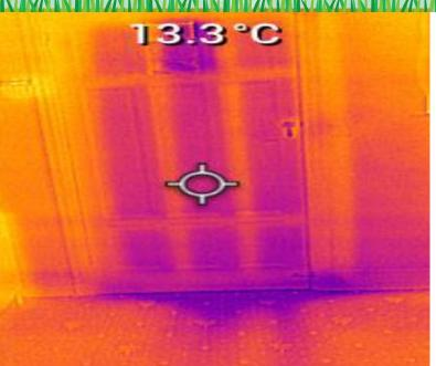
Curtains provided some degree of insulation by restricting circulation of the cooler air.
