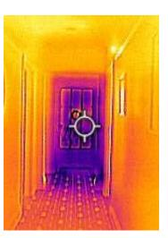
With an Infra-Red camera, you can literally see where the heat is escaping. The photos above are infrared images of a door taken from outside and inside. In a thermal image, yellow shows hotter areas and pink/purple the cooler areas.
